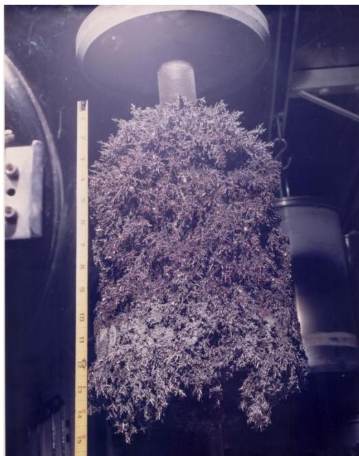
Figure 8-6. Dendritic deposit of uranium on solid cathode
